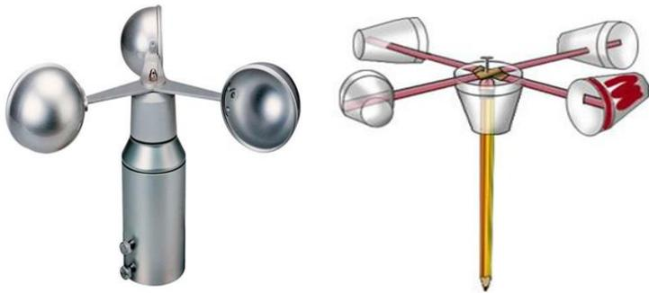
The anemometers are devices to measure the speed of wind.
